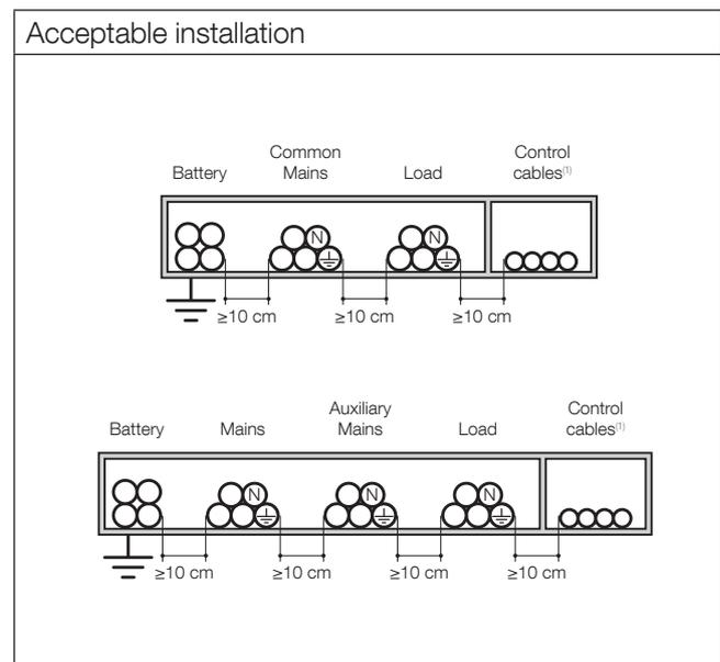
1. Control cables: connections between the cabinets and each unit, alarm signals, remote mimic panel, connection to the BMS (Building Management System), emergency stop, connection to generator.
