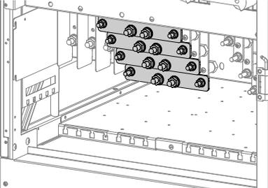
A technical line drawing showing the internal terminal block of an 80 kVA UPS. The terminal block is a horizontal assembly with two rows of terminals. The top row contains 12 terminals, and the bottom row contains 12 terminals. The terminals are arranged in a 2x6 grid. The drawing shows the terminal block mounted on a metal frame with various mounting brackets and screws. |
