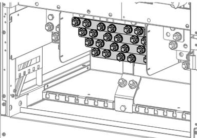
A technical line drawing showing the internal terminal block of a 120 kVA UPS. The terminal block is a horizontal assembly with two rows of terminals. The top row contains 12 terminals, and the bottom row contains 12 terminals. The terminals are arranged in a 2x6 grid. The drawing shows the terminal block mounted on a metal frame with various mounting brackets and screws. |
